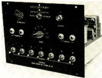
Fig. 3. Front panel view of the radio switch box, schematic diagram of which is shown in Fig. 4.
